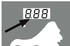
Mode 1 is the PID mode on the alpha controller. This will hold steadier temps and a more stable fire. This mode operates off of a feed rate that the user can adjust (although most will not need to). If you find the grill is consistently running hotter than your set point you can lower the feed rate. If it's running consistently colder than your set point you can raise the feed rate. Always make small adjustments when tuning your grill.
